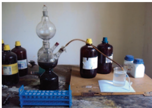
Fig. 6.12 Experimental set up for the determination of metal bioaccumulation in the isolates at H_2S gas exposure
